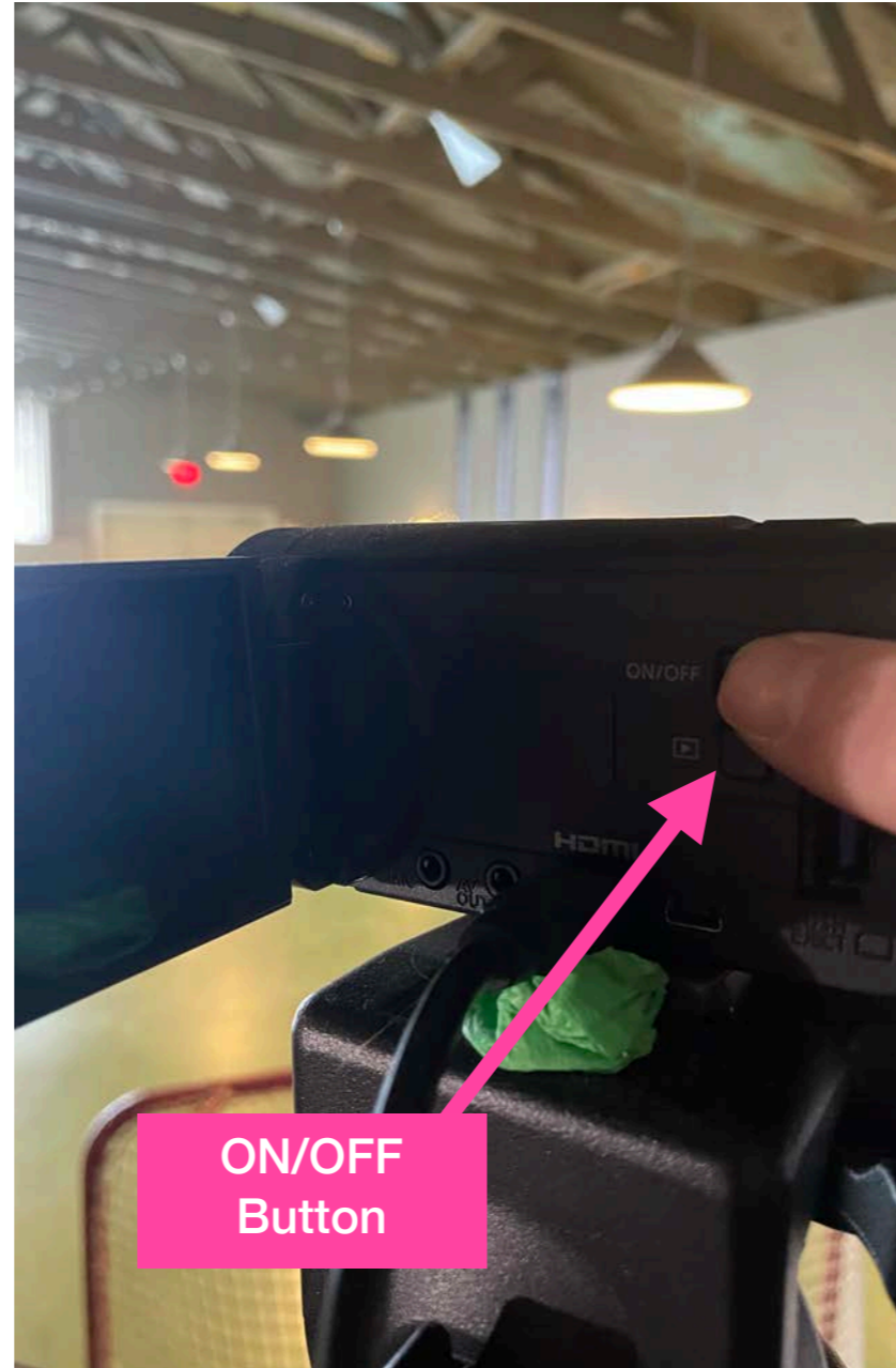
Power up the camera using the ON/OFF Button on the side.
