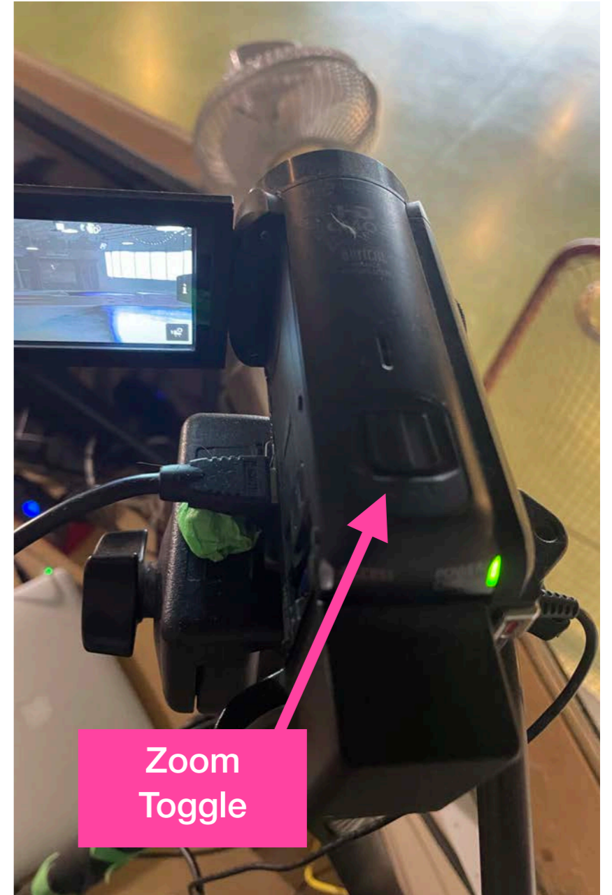
To Zoom in/out use this Toggle on the top of the camera. Push right gently to Zoom in and gently left to Zoom out.
